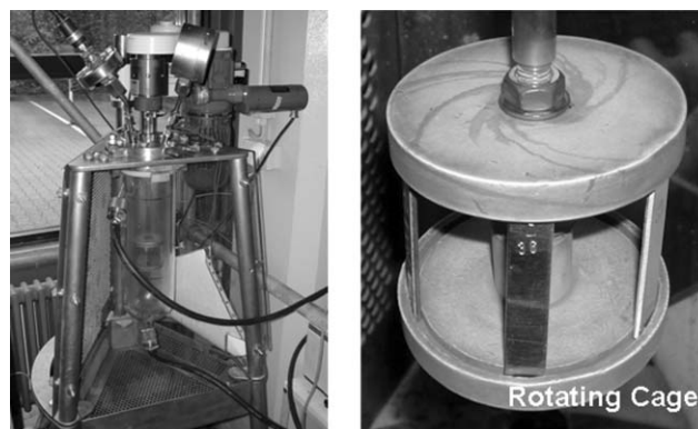
Fig. 2 Experimental setup of rotating cage experiments.
